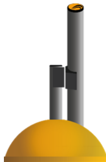
Figure 4: Angled magnetic element (Cone + angled mount + magnetic rod (MCD))
