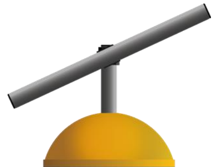
Figure 5: Angled magnetic element (Cone + angled mount + magnetic rod (MCD))
