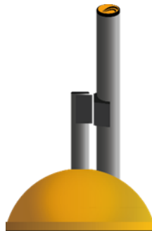
Figure 2: Angled magnetic element (Cone + angled mount + magnetic rod (MCD))
