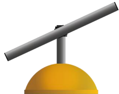
Figure 3: Angled magnetic element (Cone + angled mount + magnetic rod (MCD))
